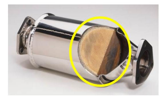
382. If excess oil enters into the catalytic converter, the conversion process is disrupted. Excess oil will coat the working surfaces of the ceramic honeycombs so that the platinum, rhodium and palladium cannot react with the toxic exhaust gases. This is called "catalyst poisoning" and the result is that the vehicle will release higher levels of harmful emissions.
